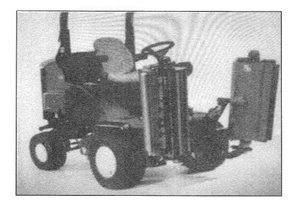
Photo no. 5 Toro LTF3000 with out-front mowers attached.
